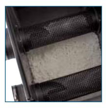
Hel-X ensures optimum media circulation Original Hel-X biomedia are highly effective at degrading pollutants in the moving bed process.
